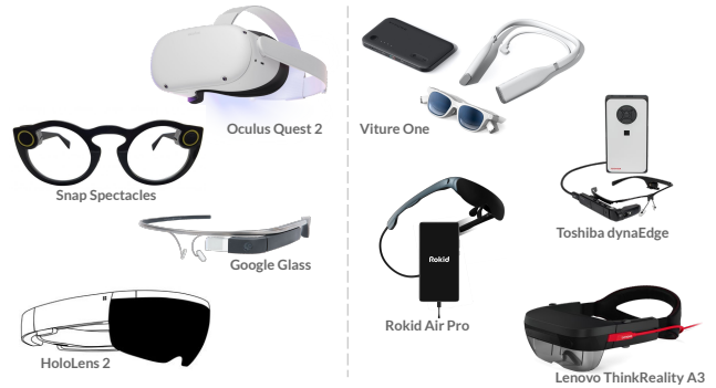
Figure 1: AR systems today are being developed either as a standalone unit with all sensors and computation present onboard, or with a companion device such as a smartphone to offload computational tasks.
